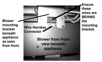
**Figure 8.23** Beneath the appliance from its front side, ensure that all wiring is moved behind the blower mounting bracket which already comes installed on the bottom of the appliance. Complete blower mounting by inserting two screws through the blower into the mounting bracket. Make the wire harness connection.
